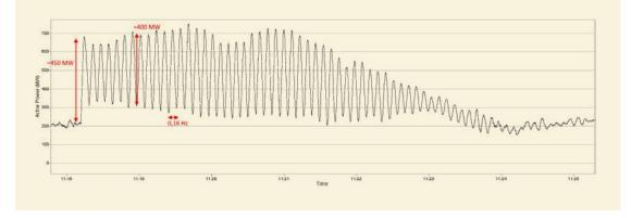
Figure 2. Active power record on the Baixas-Vic 400 kV line. Incident on 1 December 2016
