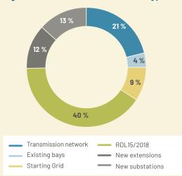
Figure 49. Breakdown of connection types of renewable energy sources in the study scenario
