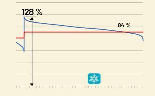
Gain factor. This is the ratio between the transmission capacity of the DLR and the seasonal capacity, calculated in aggregate for all the hours of a station in which the transmission capacity implementing DLR is greater than the seasonal capacity. The higher the ratio, the greater the capacity increase achieved when DLR is implemented.
