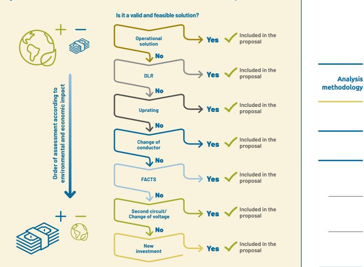
Figure 29. Flowchart for the selection of alternatives for the resolution of network problems
