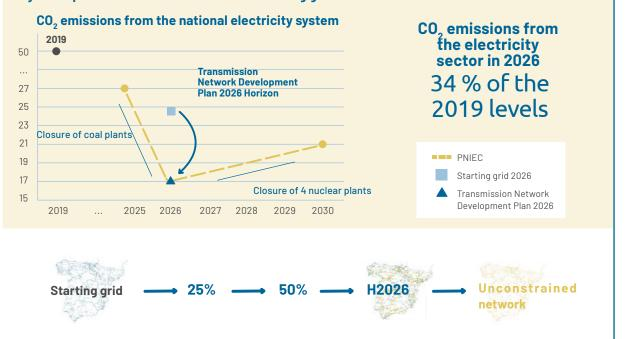
Figure 36. Estimated evolution path of the  $CO_2$  emissions of the national electricity system: planned network for H2026 vs. starting grid
